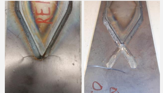
Fig 01: Fish tail technique provides 5 times higher fatigue strength
